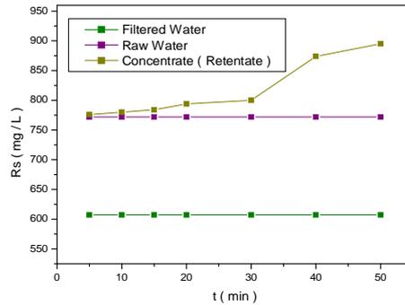
Figure 6. Variation of the dry residue according to the time of filtration
